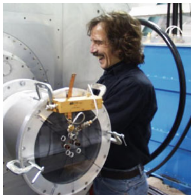
Daniel Birs in 1998 working at the Lawrence Berkeley National Laboratory on beam breakup instability impedance measurements of DARHT-II cells
