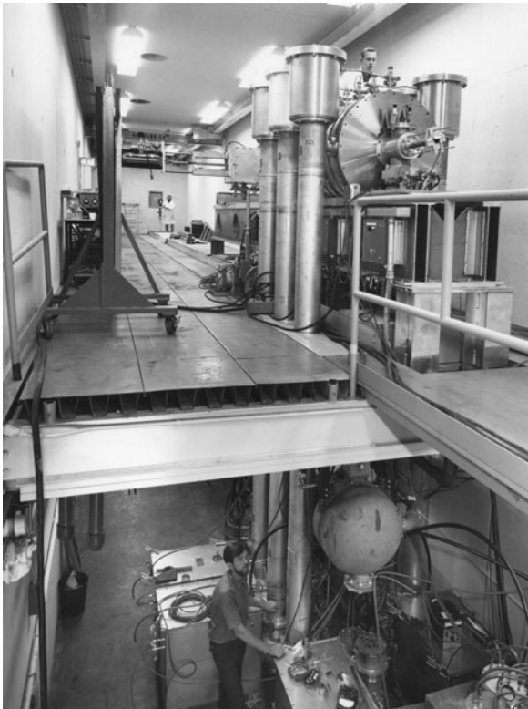
Fig. 2.3 Electron Ring Accelerator Injector, the first induction linac to use ferrite cores (1970)
